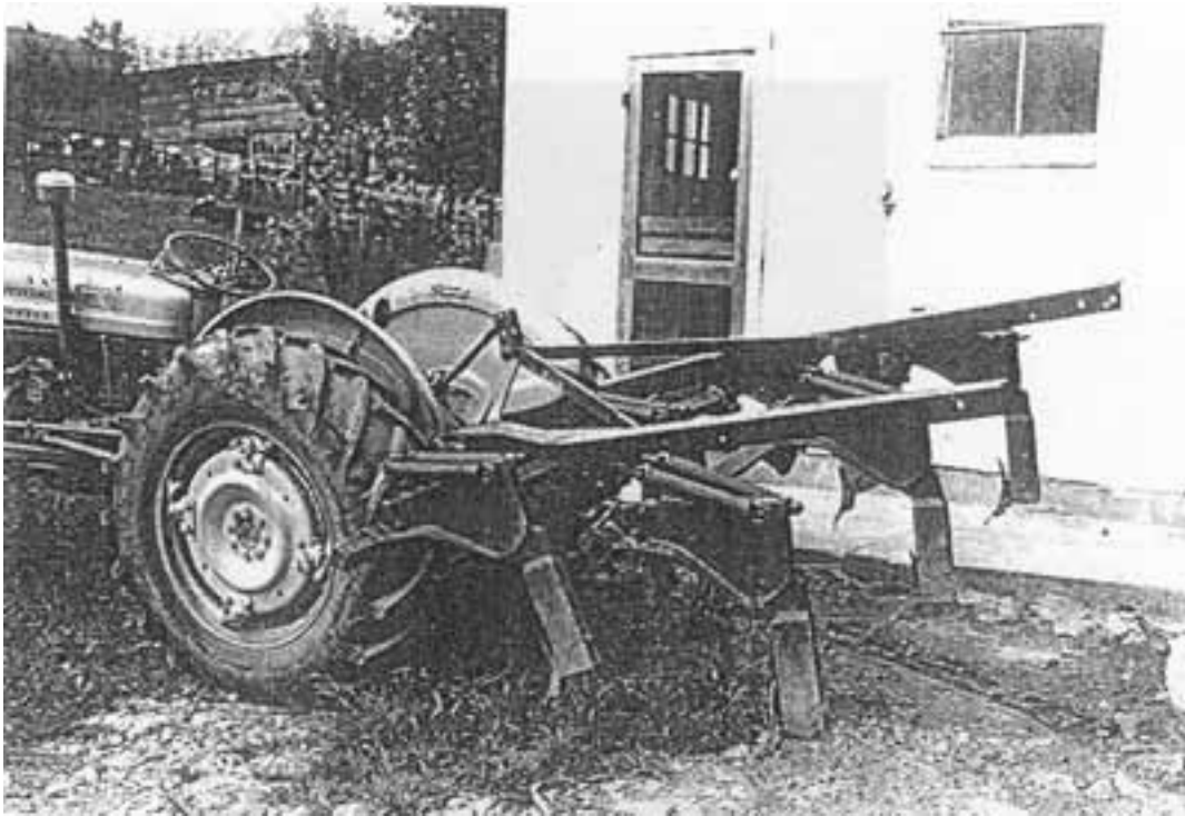
Figure 1. In 1962, Haywood County farmer John Kirkpatrick used this homemade unit to prepare a narrow, tilled zone which was later followed with a regular planter. Erosion control on a steep slope was a major goal.
