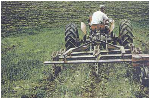
Figure 3. Early innovations and several farmers’ adaptations of planting equipment for use under no-till conditions.
